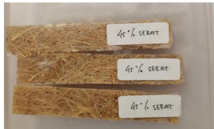
Figure 1. Coconut Fiber Composite Specimen (Personal source)
